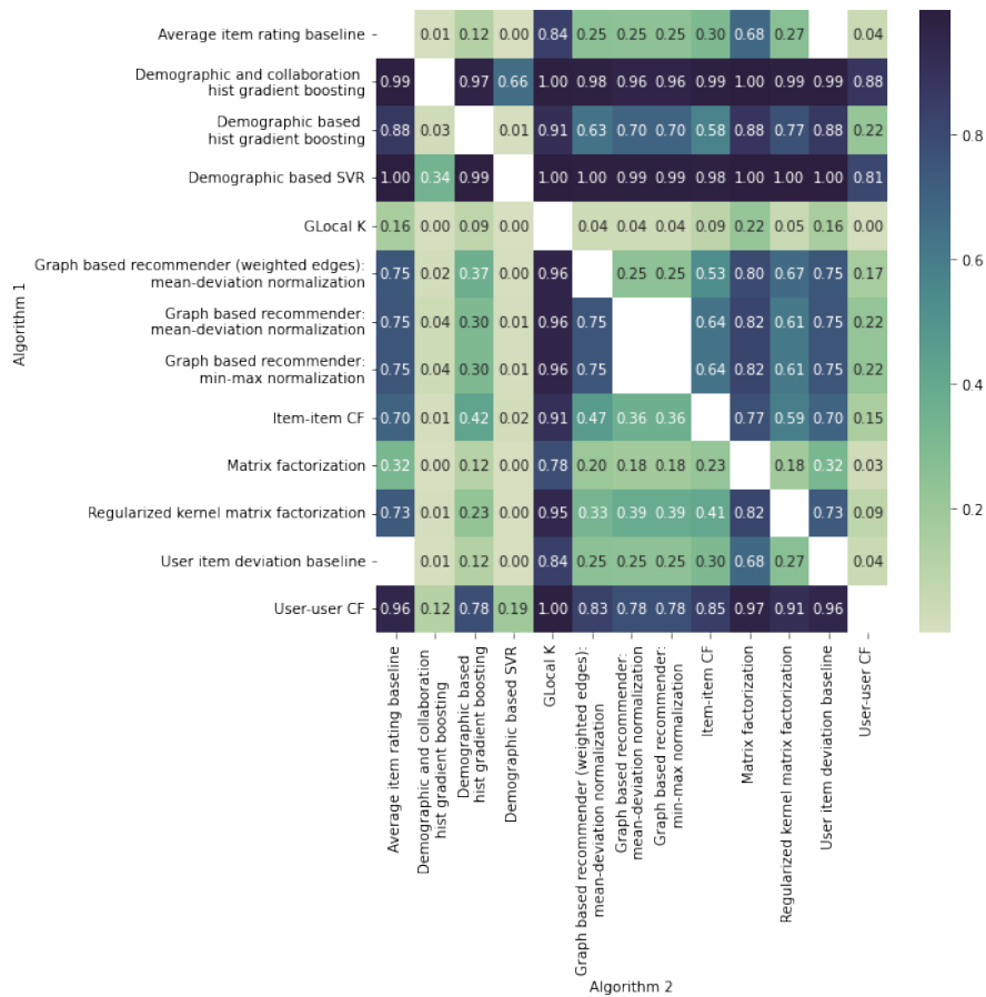
Figure 4.4: P-values from Wilcoxon signed ranked paired tests for the null hypothesis that the mean of the two algorithms is the same and hypothesis 1 that the mean of precision at k=3 for algorithm 1 is greater than metric of algorithm 2 at visitor path depth of 12
